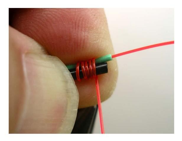
The wraps are done. Make the wraps tight but not too tight that make it difficult to pull out the tool. It is much easier to work with smaller wraps after the tool is pulled out.
