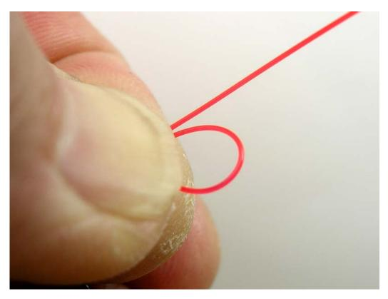
This is after the tool has been pulled out. Notice the loop. This must be pulled through quite tight to hold the wraps. The tag end of the loop (photo below) when pulled will tighten the front of the wraps. The other end(the straight on above) when pulled will tighten the back 3 wraps.
